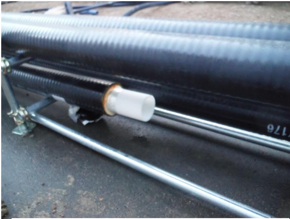
Open end of the branch pipe which caused the leakage
